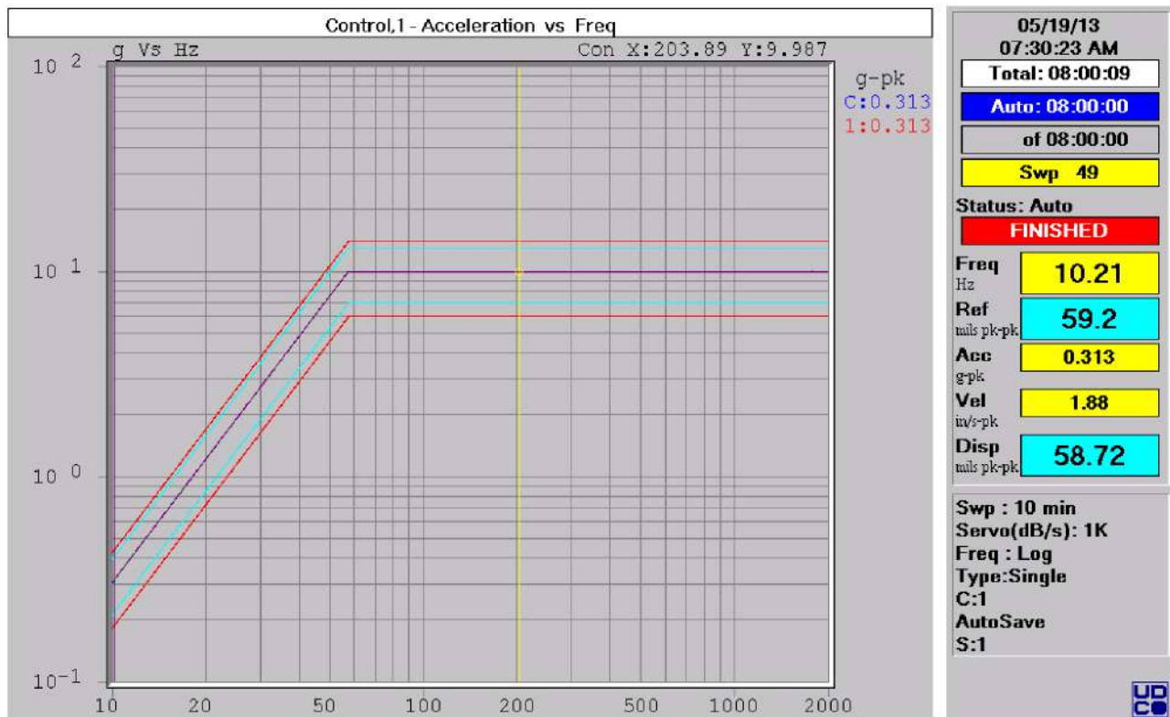
Figure 10.1.2: Sine vibration profile for testing, purple trace: ideal excitation
